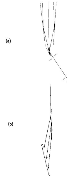
Fig. 3. (a) Schematic showing how a convergent section of supermirror guide can be used in conjunction with a multiple piece graphite monochromator to increase the wavelength spread of the incident beam in a reflectometer; (b) a specularly reflected polychromatic beam incident on a series of multilayer monochromators of different spacings and/or angles, each set to reflect a particular band of wavelengths onto a different section of a position sensitive detector as discussed in the text (from ref. [5]).
